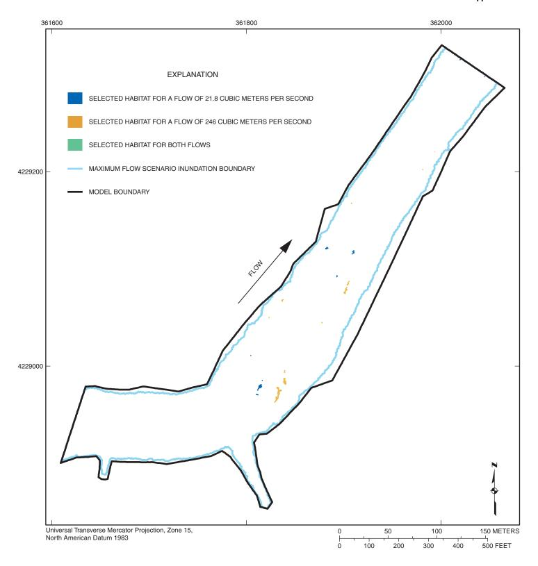
Figure 3-78. Selected habitat area distribution for habitat categories 16, 17 combined (channel catfish) at flows of 21.8 and 246 cubic meters per second at Marais des Cygnes River site MDC1.
